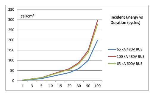
Figure 3: Software modeling analysis results for arc-flash testing
