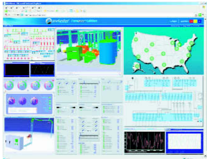
Image Two: After a Power Analytics system is deployed, thousands of arcane electrical components making up a data center’s power systems infrastructure can be presented in easily understood charts, graphs, and diagrams depicting only relevant information for specified users.. including the economic impact of operational decisions.
