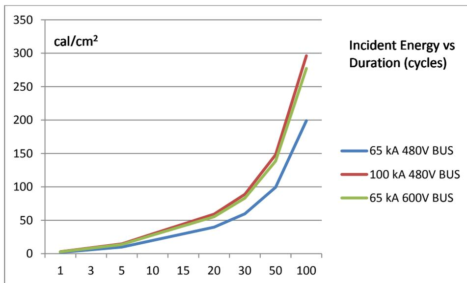
Figure 3: Software modeling analysis results for arc-flash testing
