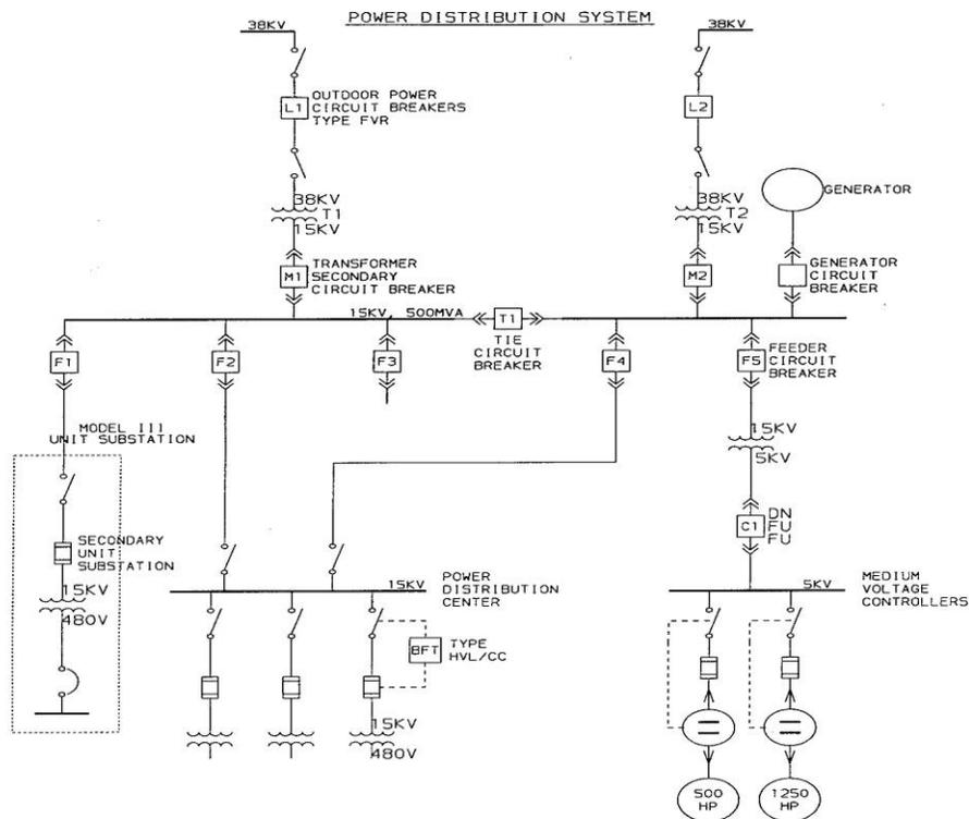
Figure 1: Typical One-Line Diagram
